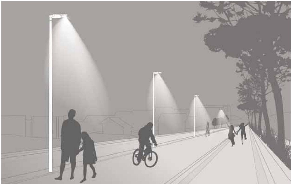
Image showing how illumination is controlled and directed downwards
