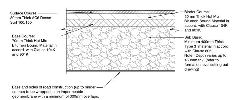
Carriageway - Permeable Tarmac (Full Depth) (C.B.R. 3-5) Total Construction Depth = 550mm (min)
