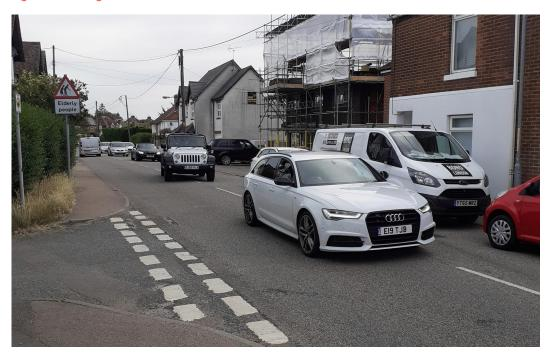
Section 1c runs between Maple Close and the Rough Common Village Hall. This sub-section features a carriageway width of approximately 6.3m. An inset parking bay is provided outside of properties 95-101 (Figure 8). A separate unpaved service road then feeds properties behind a small green area adjacent to the junction with Church Wood Close.
