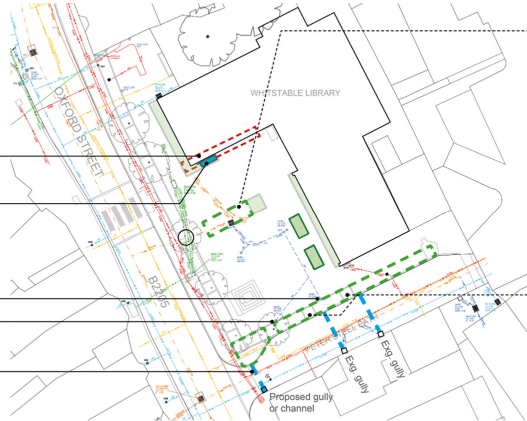
Raingarden with amended drainage connection - diverts surface water run-off into SuDs with overflow back to existing below ground drainage.
