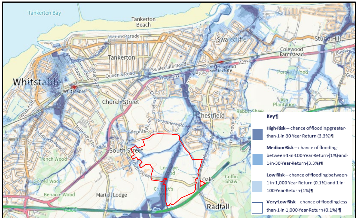
Figure 2-1: EA Long Term Flood Risk Maps – Flood risk from Surface Water (Gov.UK website)
