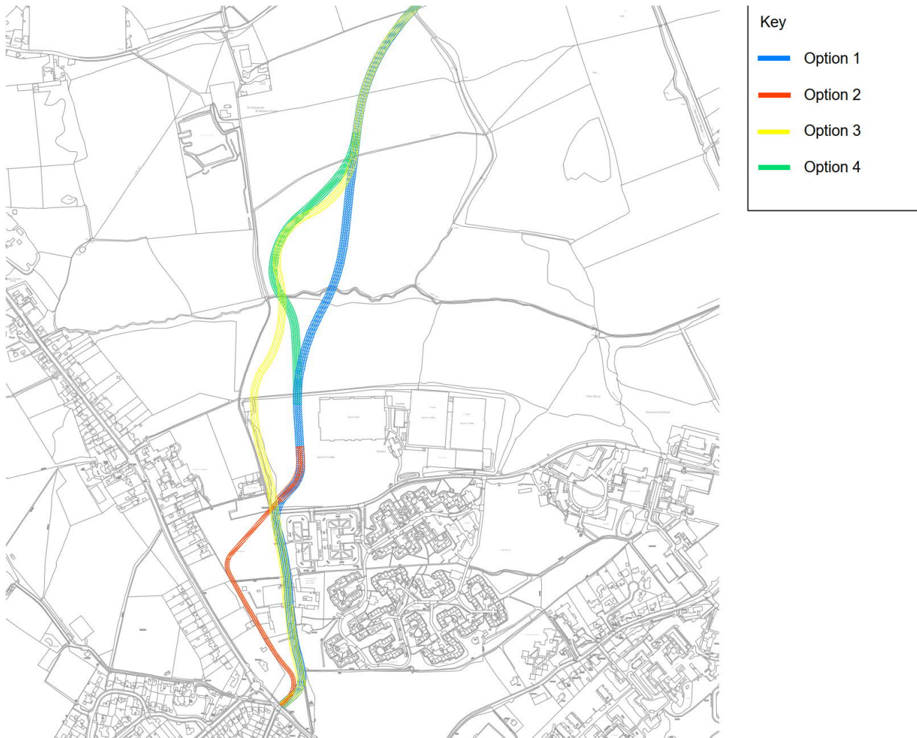
Figure 2 – Access Road Alignment Options
