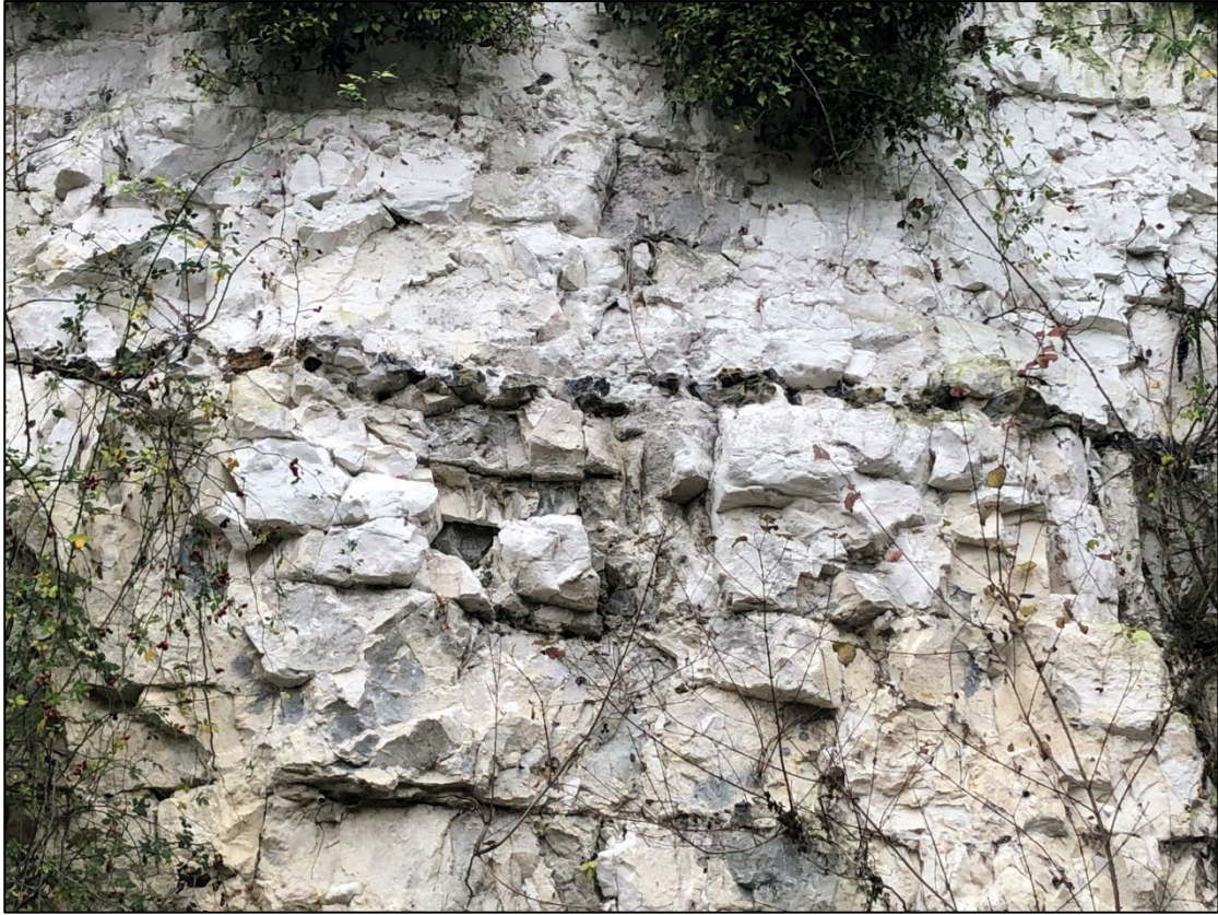
PLATE 9 – FLINT MARKER BEDS AND EVIDENCE OF ROCK FALLS AT VERTICAL CLIFF EXPOSURE
