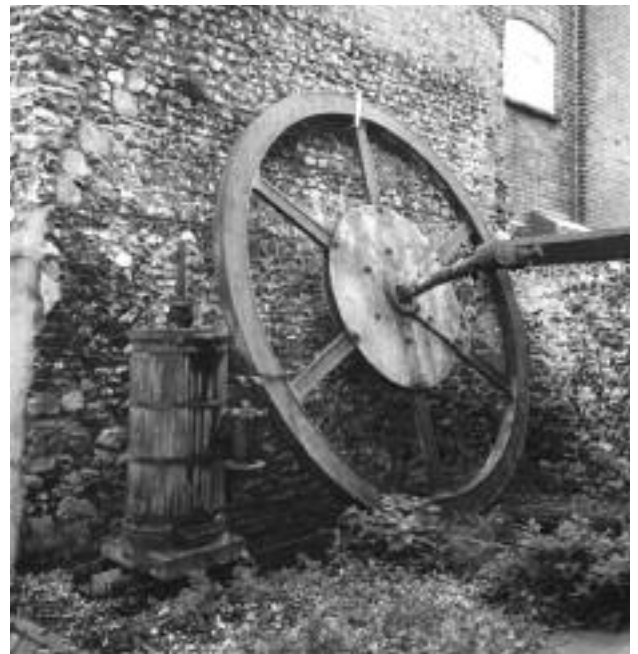
Remains of winding engine fly wheel at Canterbury Museum Store, Gas Street
