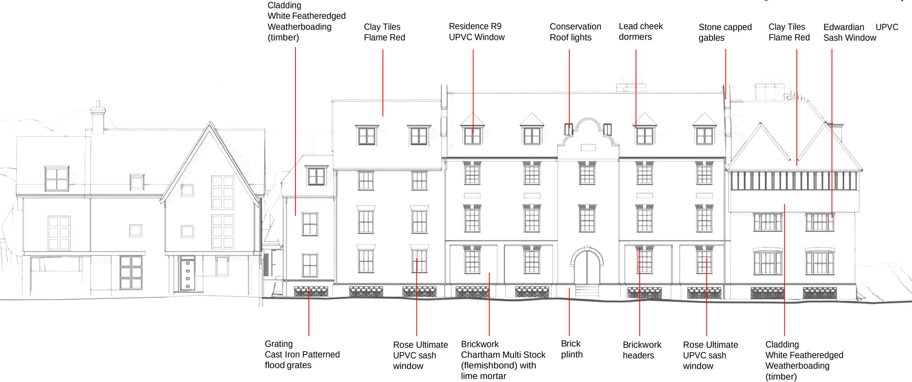
Fig. 55: Elevational Materials Study
