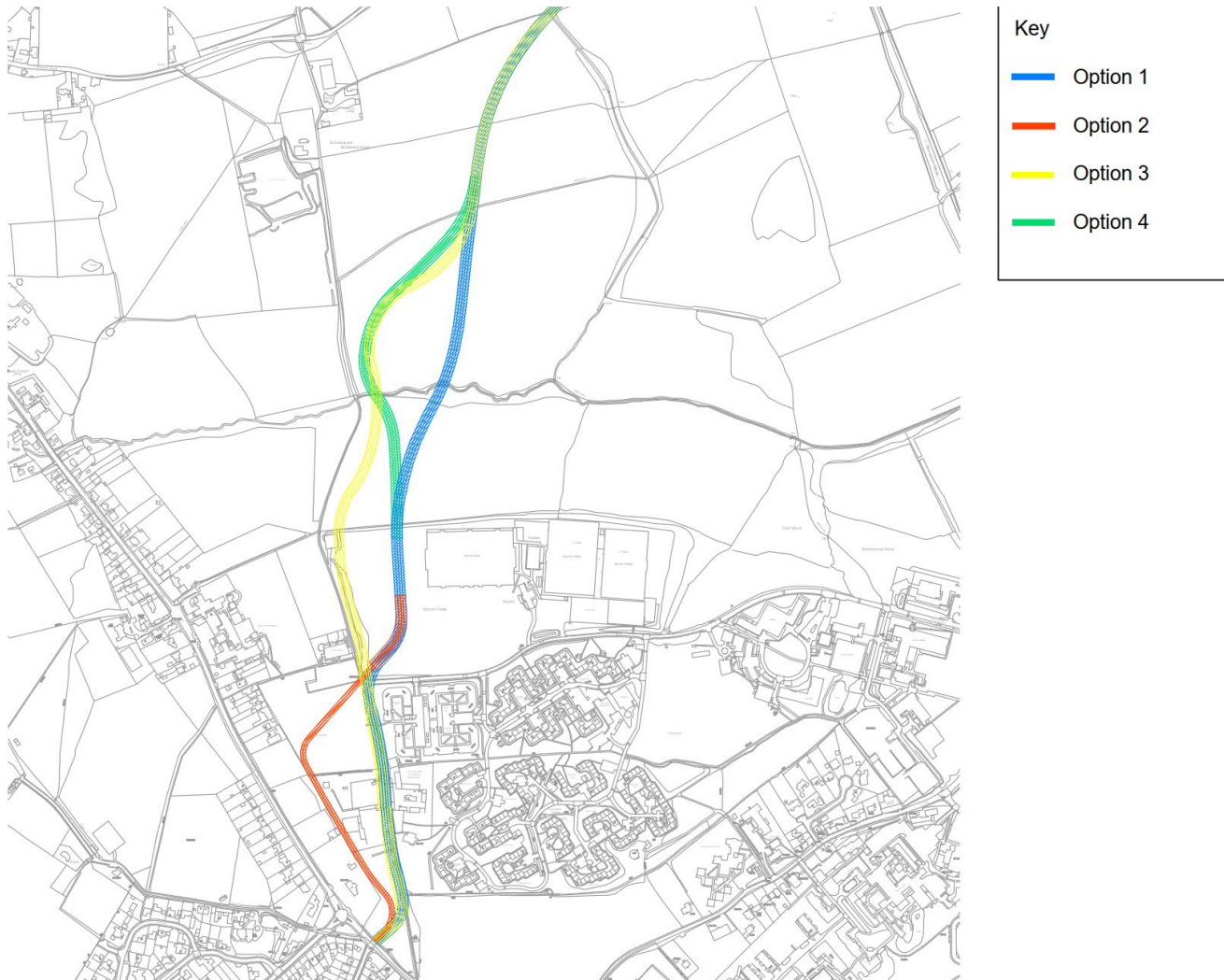
Figure 4 – Access Road Alignment Options
