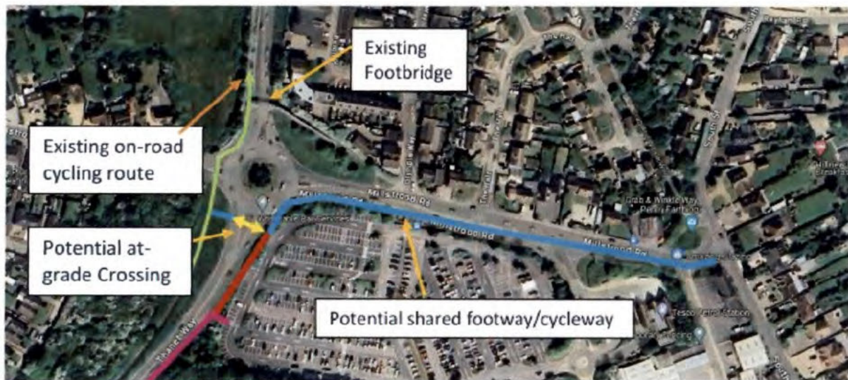
Figure 4: Extension to Millstrood Road cycle / foot path
